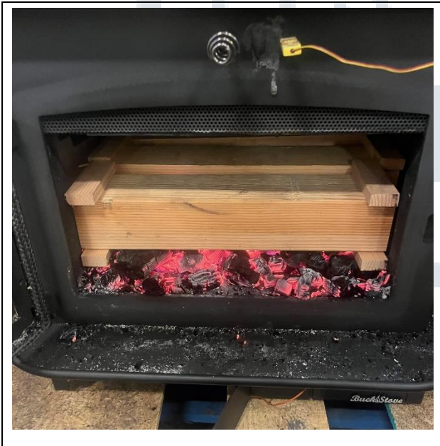
Test Fuel Loaded in Stove
