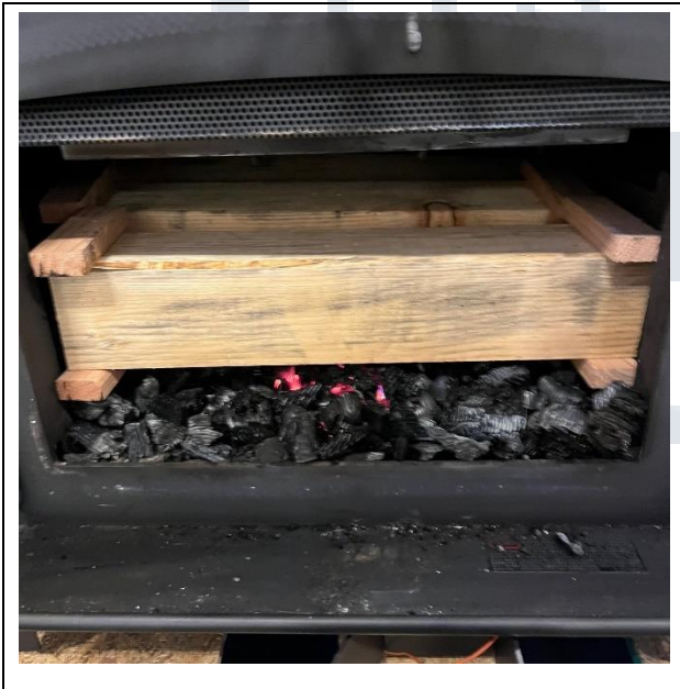
Test Fuel Loaded in Stove
