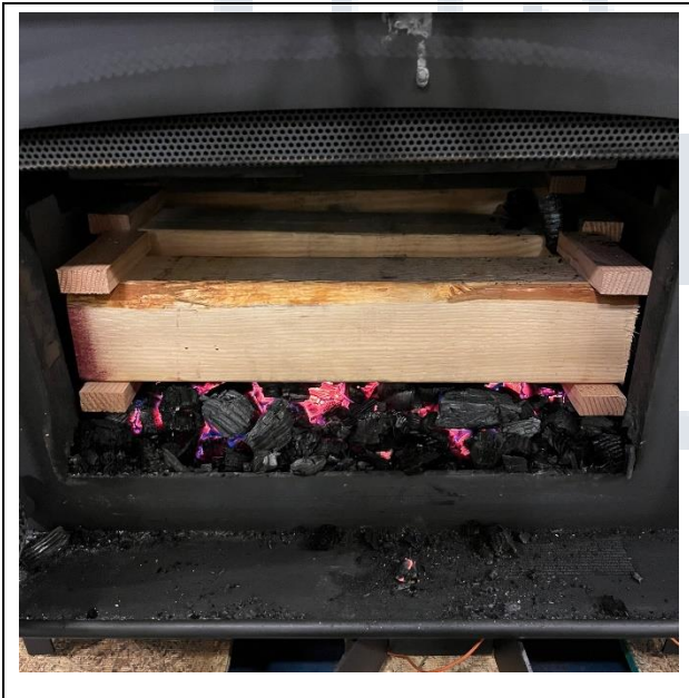
Test Fuel Loaded in Stove
