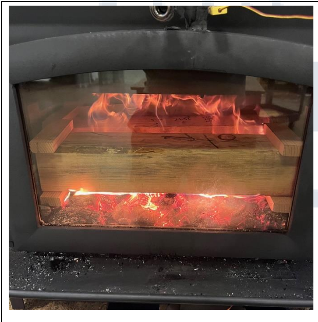
Test Fuel Loaded in Stove
