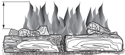
Figure 22 - Incorrect Burner Flame Pattern
